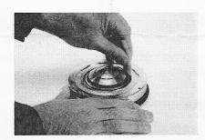
3. Visually inspect the gap and make sure that it is clean (in case of particles presence use adhesive tape wounded on a little strip to remove them). Gap must be completely free of any particle.
